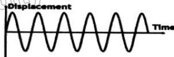
Figure 17.9 (a): Displacement-time graphs to illustrate undamped oscillations.
